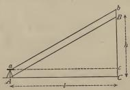
the observations give  $3^{\circ}$  07' 15'' as the probable value of the angle of elevation *bac*. From (38)' the mean correction for curv-
